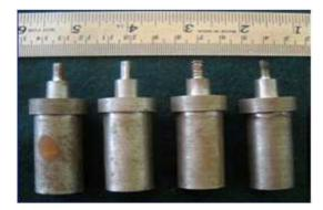
Figure 2: Different Tool Pin Profile Selected in this Investigation
